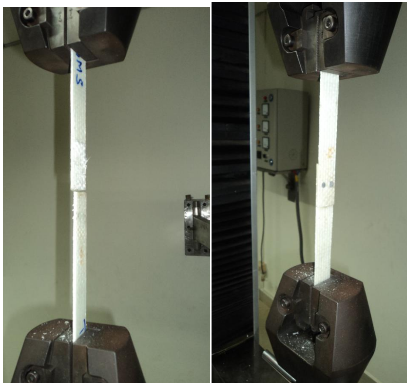
Fig. 5.5 to Fig. 5.7 Testing of Riveted Joint (Before & After)
