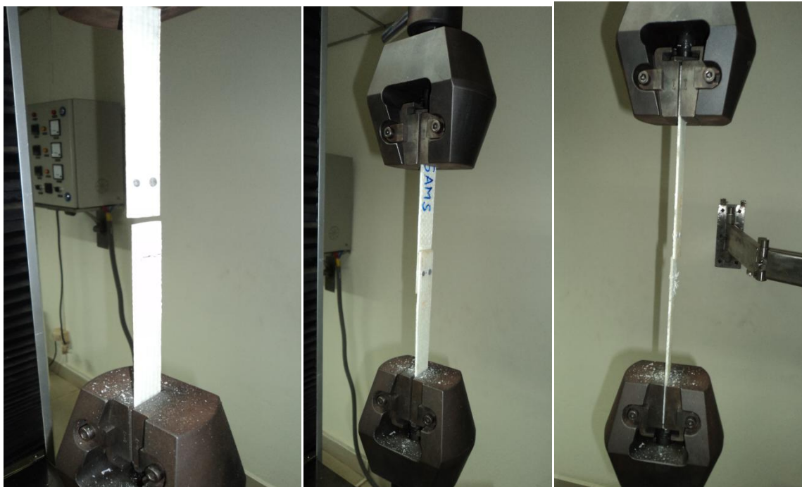
Fig 5.8 to Fig. 5.9 Testing Of Hybrid Joint (Before & After)
